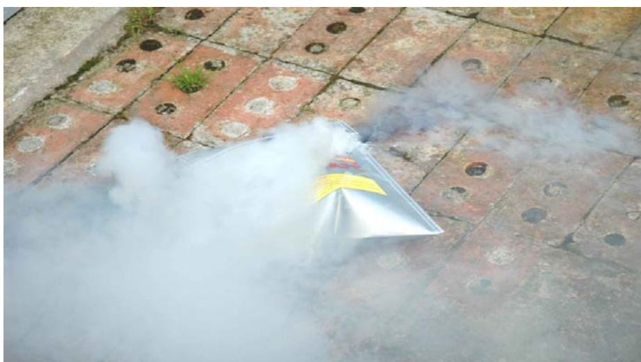
A deliberate LiPo fire using a safety sack to contain the flames.
